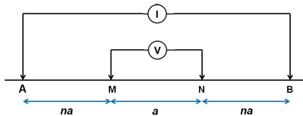
**Figure 2.** Schlumberger electrode configuration. A and B, are current electrodes, while M and N are potential electrodes
